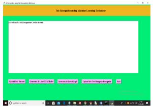
After you've loaded the dataset into the screen, you can construct a CNN model by clicking the "Generate & Load CNN Model" button.
