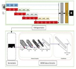
Convolution Neural Network technique (CNN) for Iris recognition system
