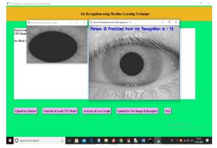
We extract the IRIS characteristics shown in the first picture from the uploaded image; CNN then used this image to make a prediction about whose person ID the IRIS belonged to (person ID 15), as seen in the upper screen. To see whether CNN can make accurate predictions, I will now upload a picture from the CASIA folder.
